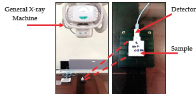
Figure 2. Setup for X-ray shielding measurement.
